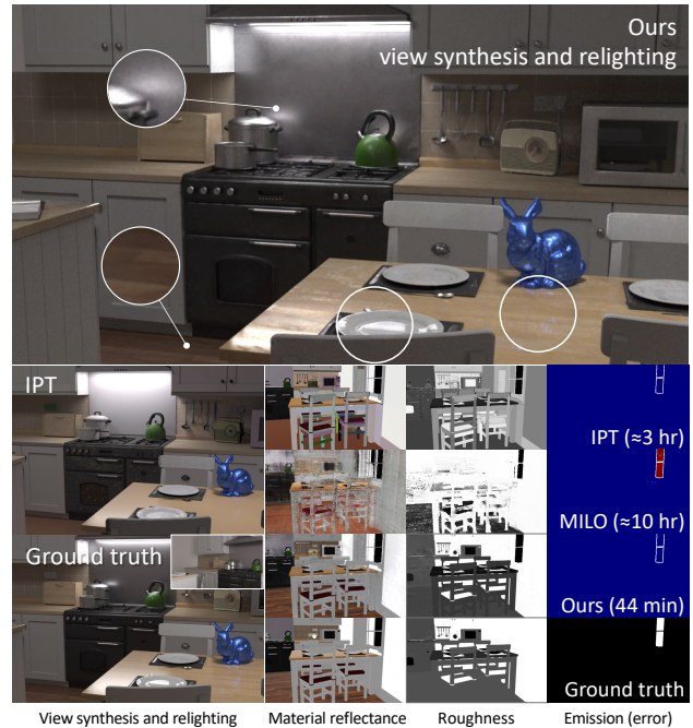
Figure 1: Ours vs standard IPT. IPT [1] takes a piecewise constant parameterization of material to reduce Monte Carlo variance and ambiguity for inverse rendering, losing fine spatial details as a result. Directly extending it to complex material representation (e.g. MILO [51]) shows very slow convergence. In contrast, we propose Factorized Inverse Path Tracing (FIPT) to get rid of variance and reduce ambiguities, yielding efficient and high quality BRDF-emission (4th row), appealing relighting (1st row), and object insertion (the bunny on the table). The presented scene is synthetic with the inset showing the input (lower-left sub-figure).
