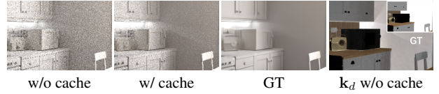
Figure 5: Diffuse radiance cache from L' helps reduce variance and error for shading estimation (2nd image). Without it, sampling the tiny emitters below the cabinet will be difficult (1st image), which leads to incorrect shading and albedo (4th image).
